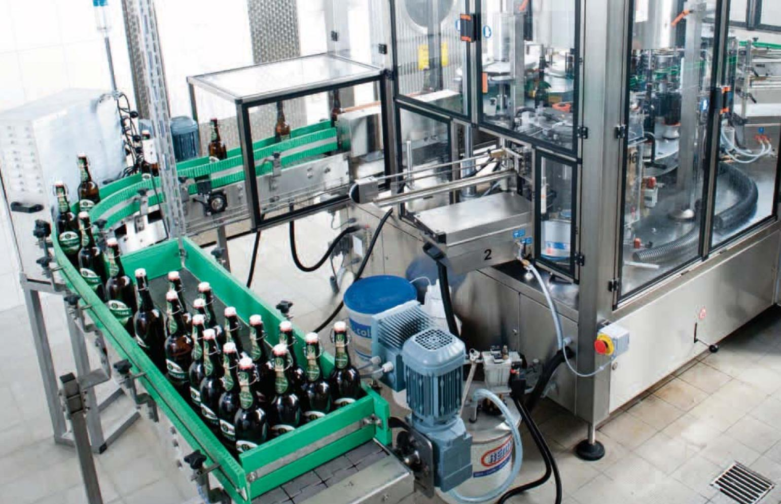
*The very compact Kosme Extra labeller features an Extrafix centring unit that enables different bottle formats to be handled up to a size of three litres.*
