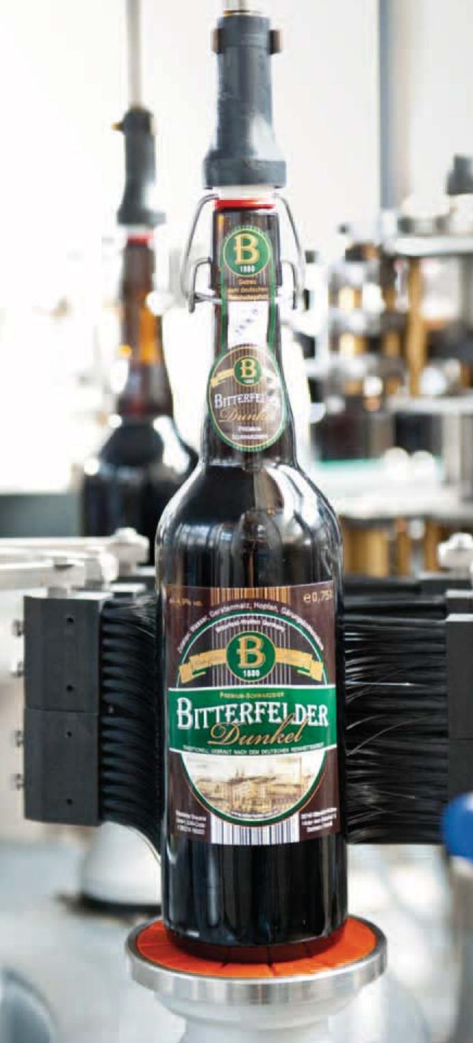
***Two original cold-glue labelling stations from Krones dress the bottle in body, back and swing-stopper tamper-evident labels.***
