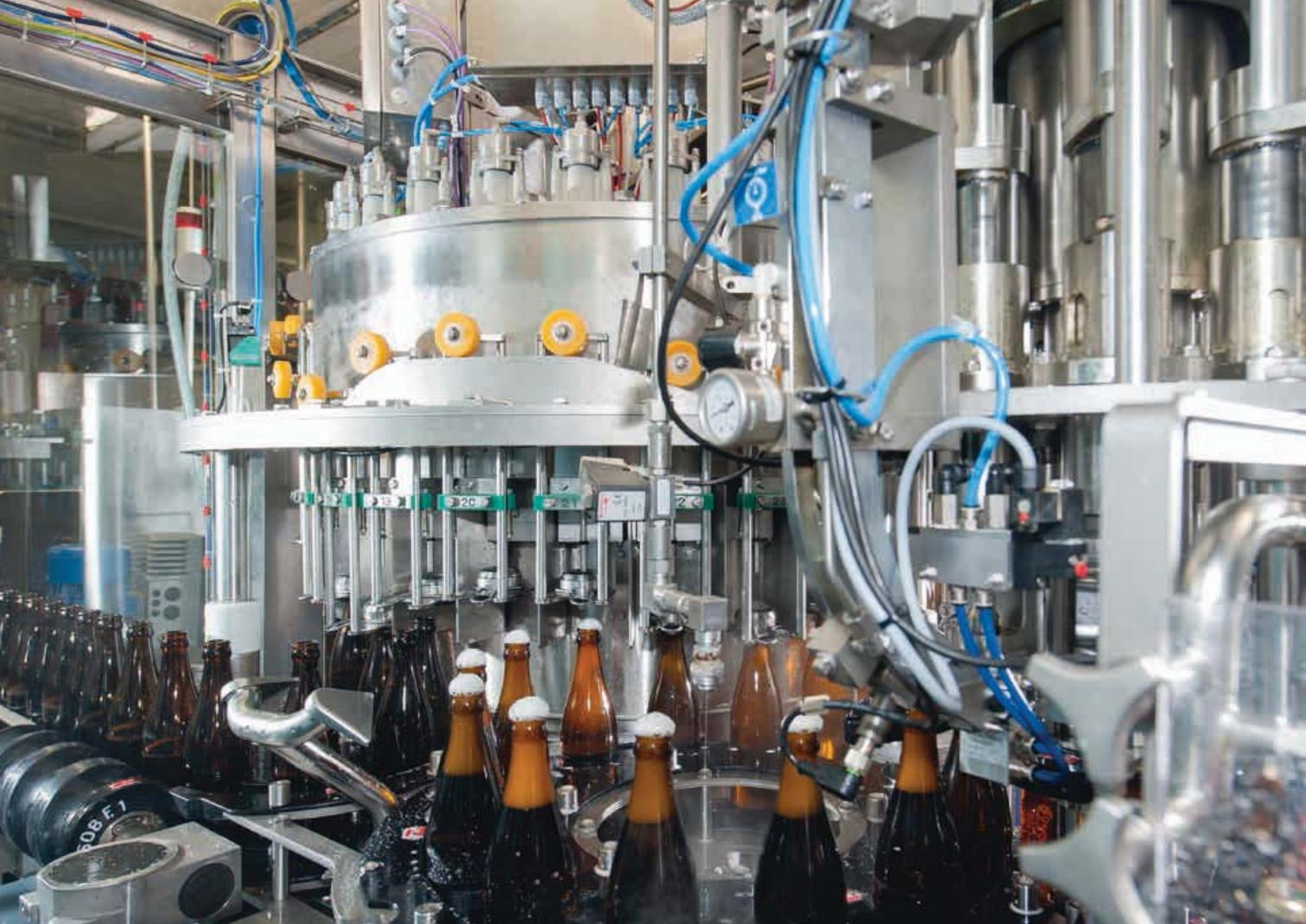
***The height-adjustable rotary Isoblock G filler from Kosme, with 28 filling valves and a pitch dimension of 960 millimetres, consists of a filling unit and a crowner turret.***
