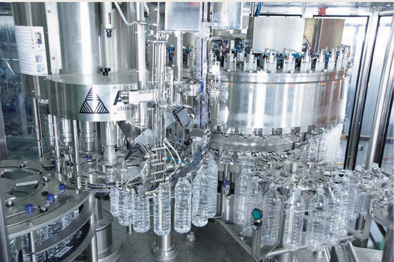
BLOC-synchronisation of the KSB 6R stretch blow-moulding machine (top) and the Isobloc NH filler (bottom)
