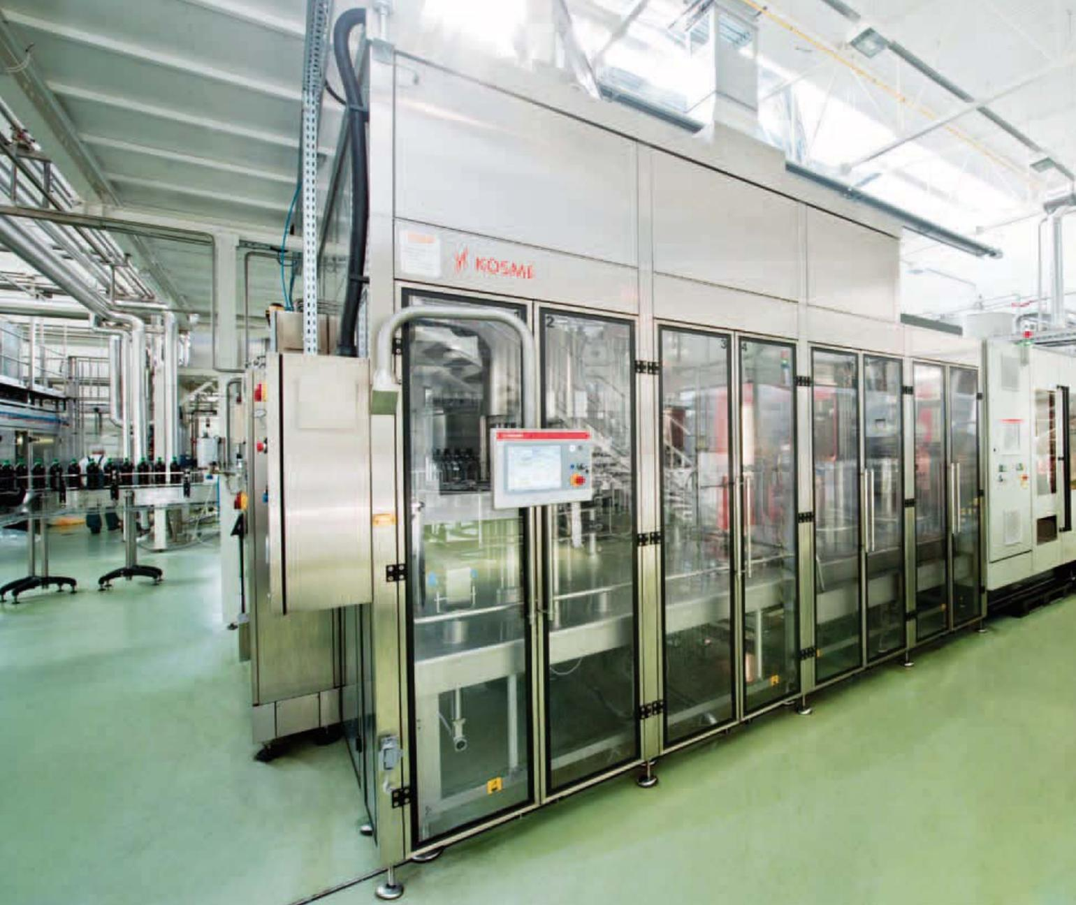
*The line incorporates a Synchronblock featuring a KSB 6R rotary stretch blow-moulding machine and a filler.*
