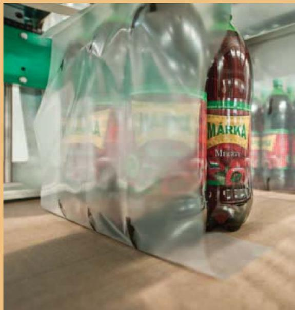
*Shrink-packs with 3 × 2 or 3 × 4 containers are packed without pads or trays and wrapped in transparent or printed films.*
