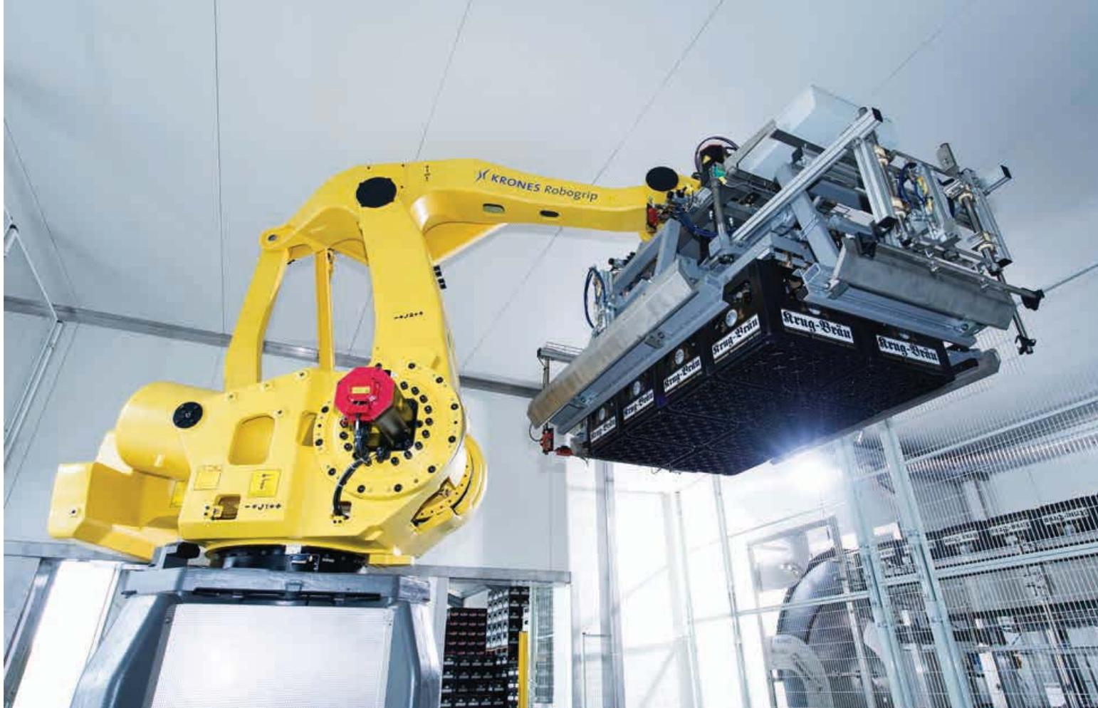
*Despite the rating, which one is inclined to call medium, Krug utilises a Robogrip palletising robot. This handles both depalletising and palletising, and at a later juncture is to load the full kegs as well.*
