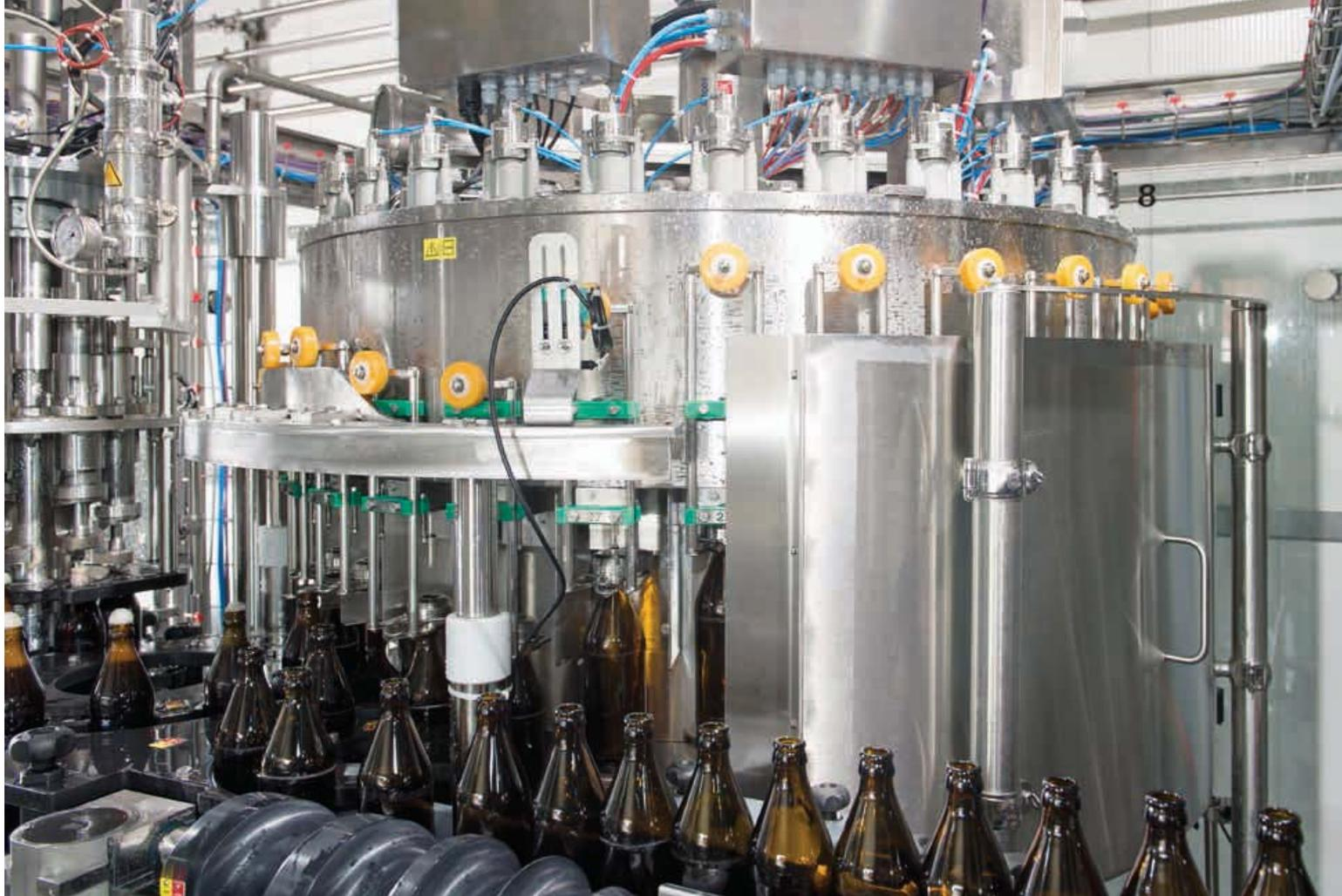
*The filler chosen by Kronen is an electro-pneumatic Kosme Barifill with 30 filling valves.*
