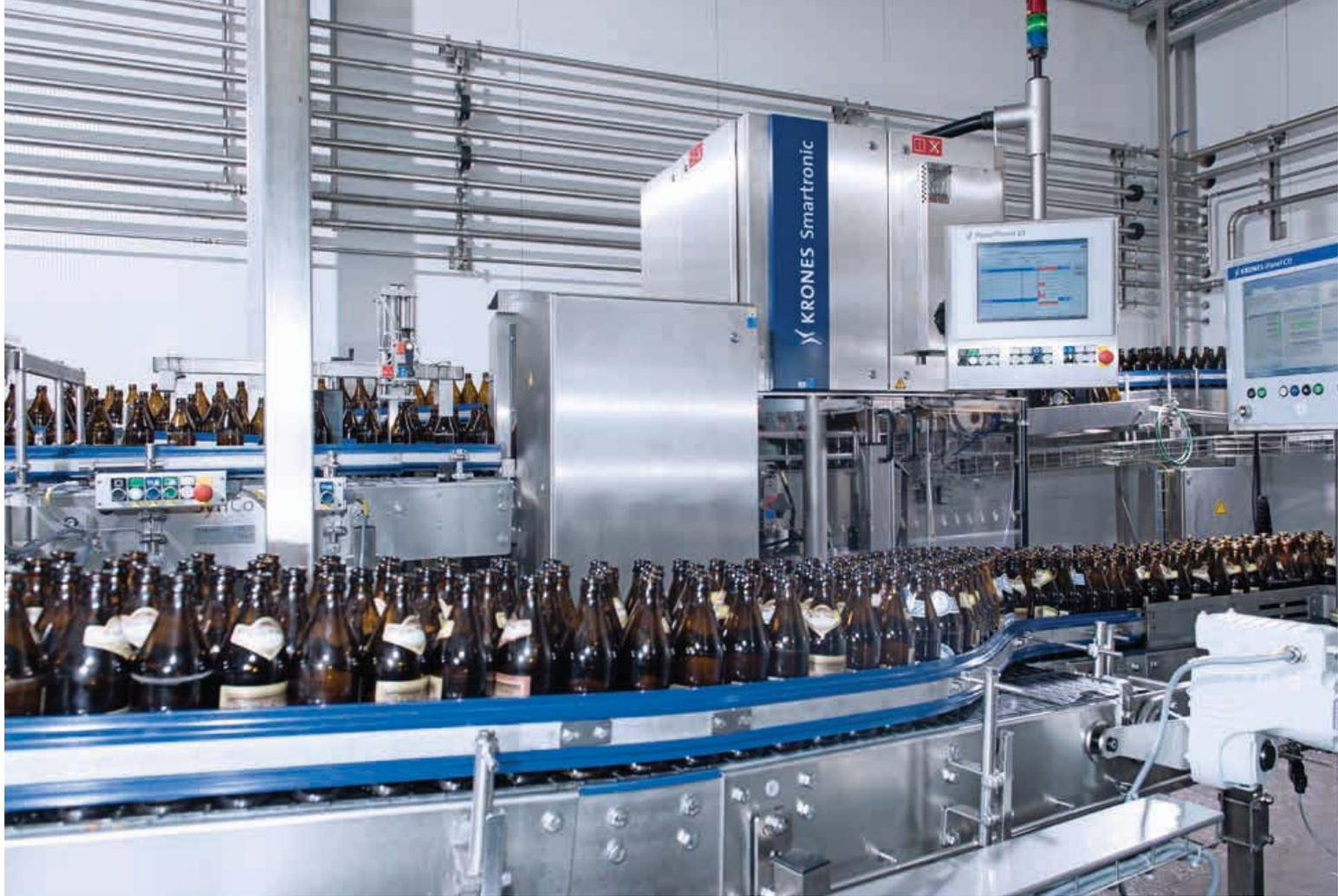
*The new line is rated at 8,000 bottles an hour and erected on a footprint of a mere 240 square metres.*
