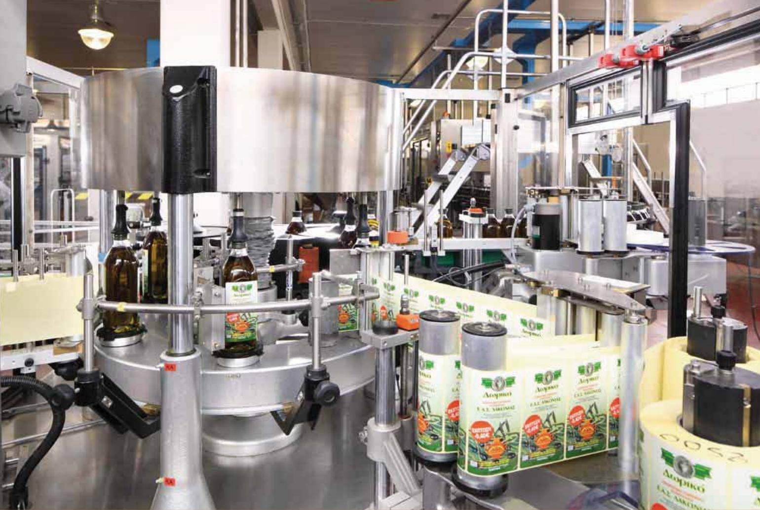
*The bottles are each dressed in a body front, shoulder and back label on an Extra AD labeller.*
