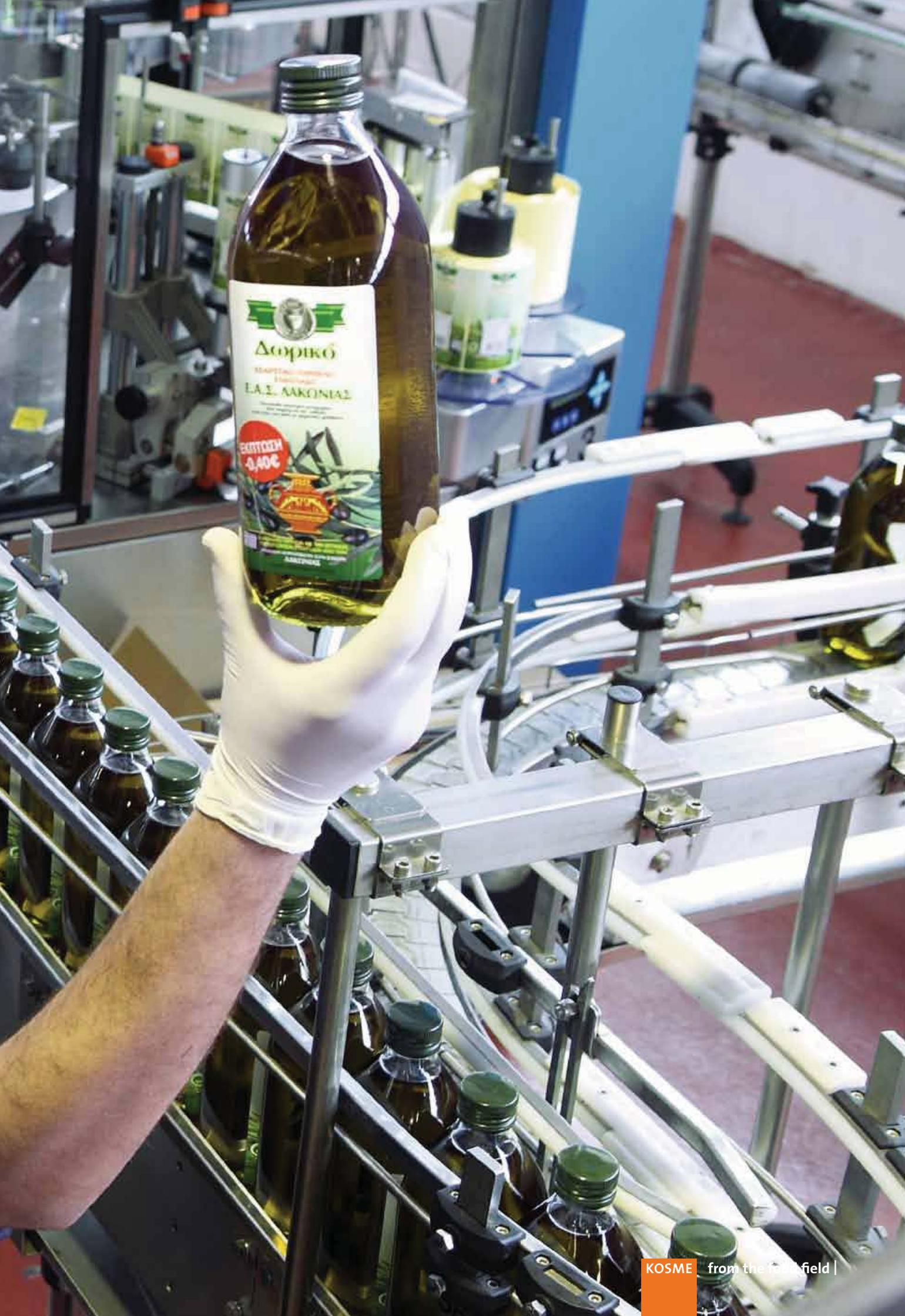
*In the Greek region of Laconia on the Peloponnese, the U.A.C. Lakonia enterprise is filling extra virgin olive oil for a network of Greek smallholders. For this purpose, the company has installed a new bottling line for glass and PET from Kosme, in addition to an existing relatively small Kosme line, plus a Kosme filler for canisters.*
