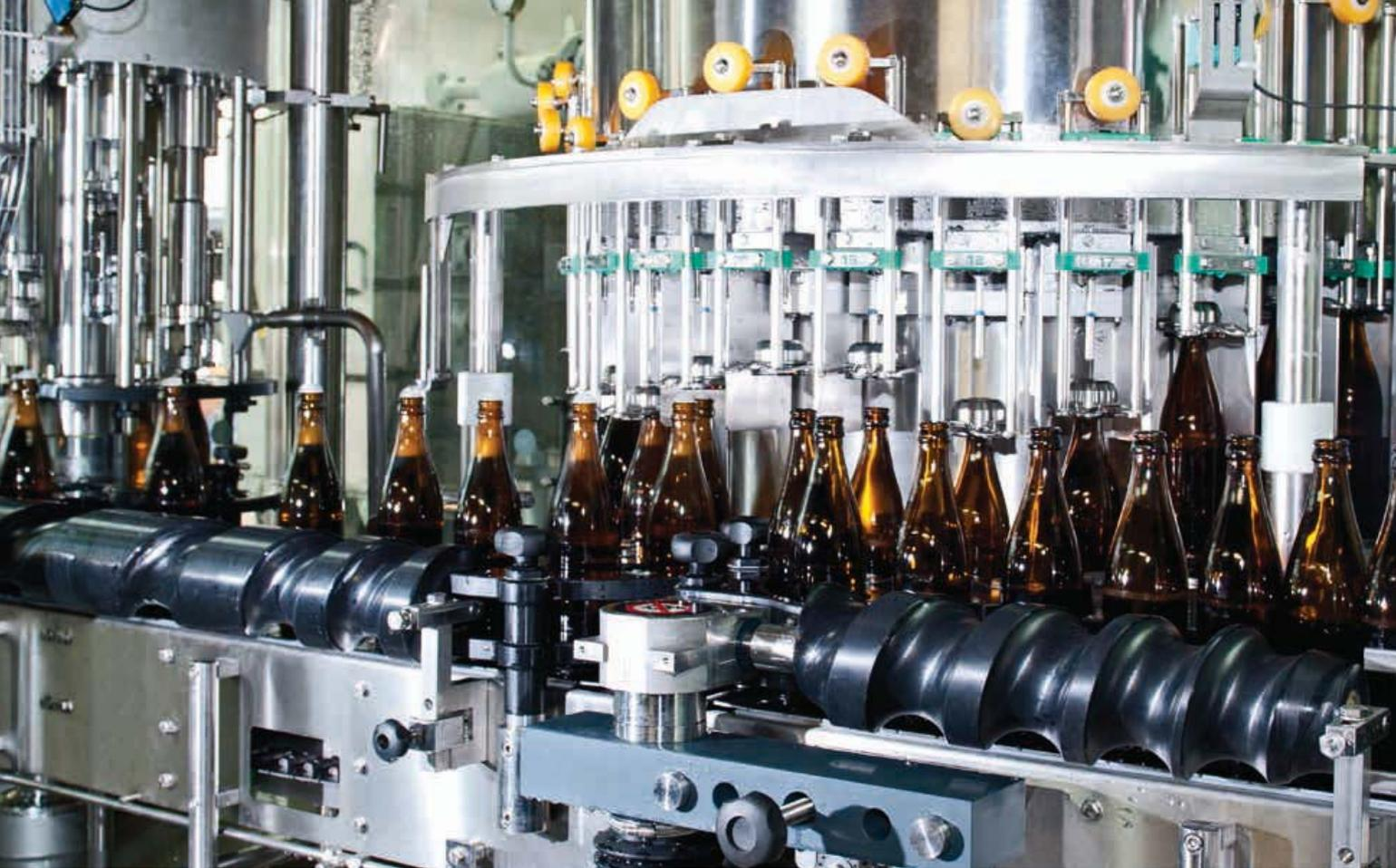
*The Barifill from Kosme, with its 28 filling valves, works with double pre-evacuation and CO<sub>2</sub> pressurisation when filling beers, thus ensuring minimised oxygen pick-up and long-term product stability.*
